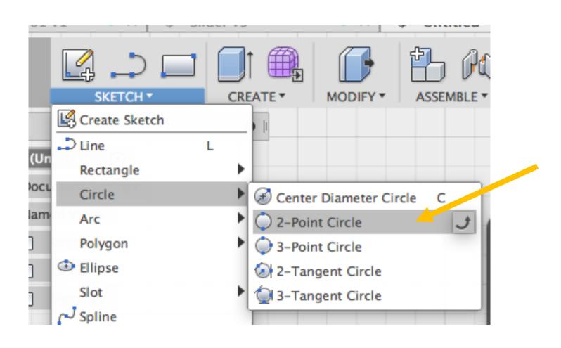
Step 38: Draw a 7mm diameter circle where point 1 & 2 sit on the bottom line of the surface as shown below.
