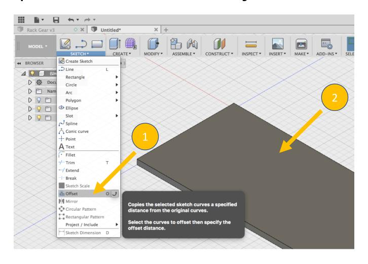
Step 29: Click on the surface's edge, then key in "-2.7mm" and hit "Enter".
