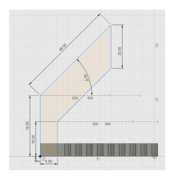
Step 24: Extrude that shape by 30mm, then save it as "STL" file. And you are done for the rack gear.
