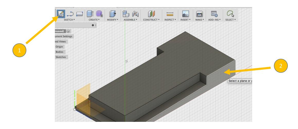
Step 36: Next, draw a 2mm horizontal line at the bottom of that surface.
