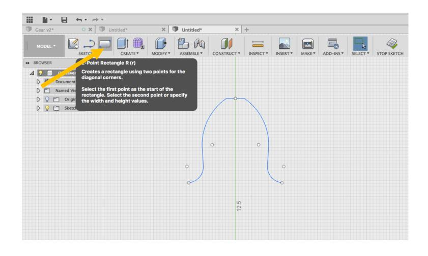
Step 14: Select the tooth's shoulder as the first point. Key in "3mm" for the height and "54mm" for the length of the rectangle.
