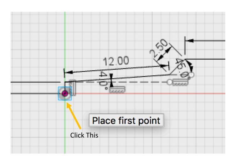
Step 19: Drag your line to right hand side. Key in "12mm" and "0 deg", then hit "Enter".
