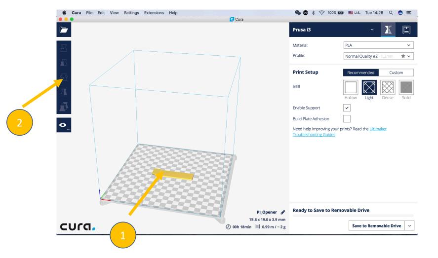
Step 72: Click and hold the red ring, then drag it to rotate the opener by 90 degrees.
