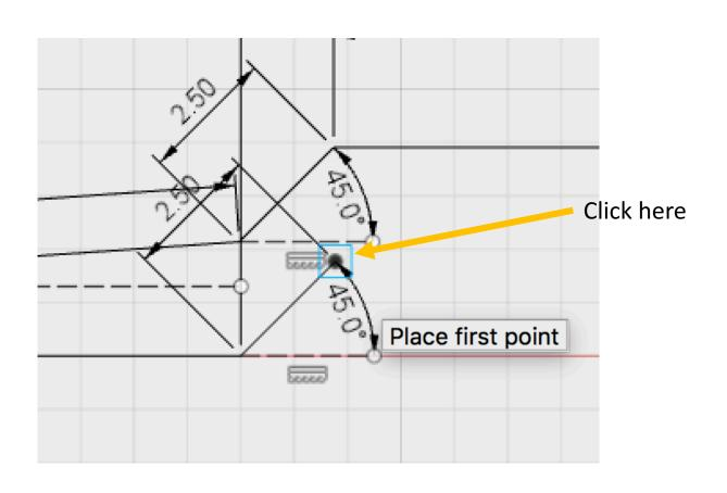
Step 23: Move the line to your right, key in "65mm" and "0 deg", then hit "Enter".
