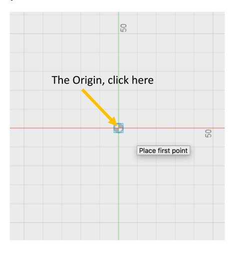
Step 5: Move your mouse to the top. Key in "1.3mm", hit "Tab", then key in "90 deg". Hit "Enter".
