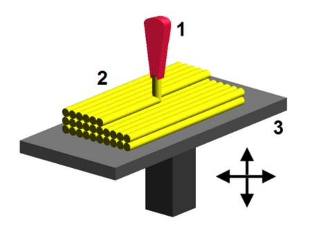
The 3D object is fabricated layer by layer with melted plastic.
